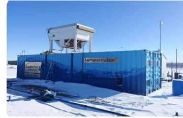
Production of NGL's and methanol from associated flare gas in North Dakota
